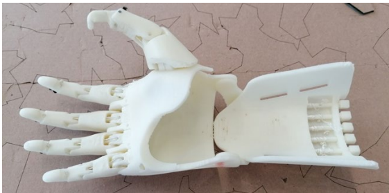
Hand-prosthesis made by Additive Manufacturing (FFF)
